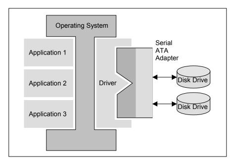
Figure 2.2 Drive system configuration
